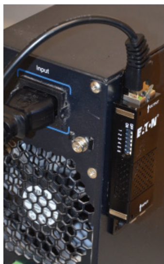
Eaton EMP Gen 2 installed on UPS
